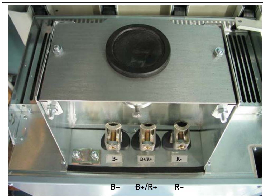
Figure 6-23. DC and brake resistor terminals on FR9; DC terminals marked with B- and B+, brake resistor terminals marked with R+ and R-
