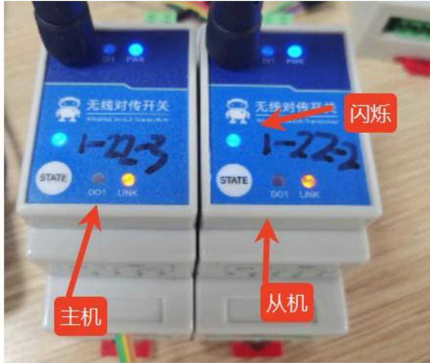
Figure 3-2-2 After the host and slave are paired successfully
