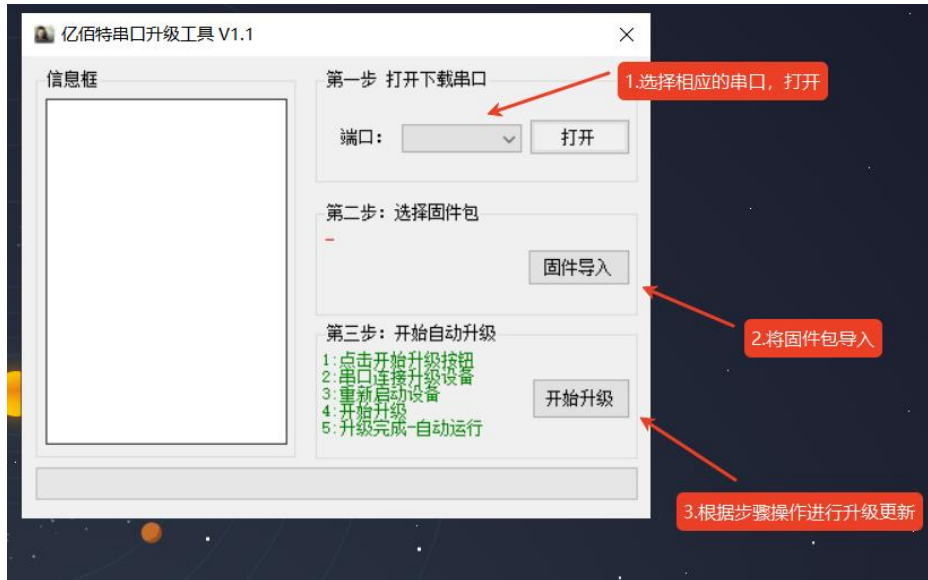
Figure 4-4-1 Firmware upgrade operation process
