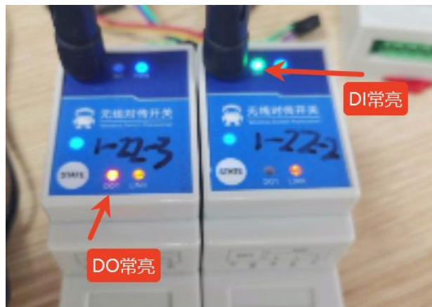
Figure 3-2-3 Slave DI controls host DO output
