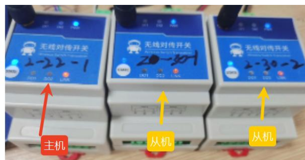
Figure 3-3-1 Schematic diagram after successful one-to-many connection
