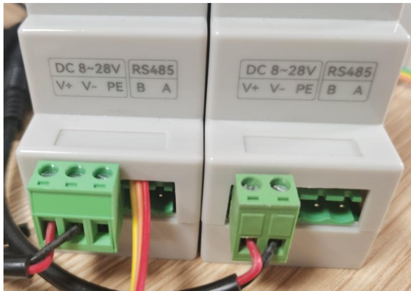
Figure 3-2-1 Power supply wiring diagram
